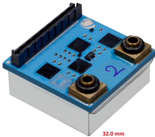
Fig. 10. Detector cube #2 with scintillator array, ASIC side with coolant connectors.
