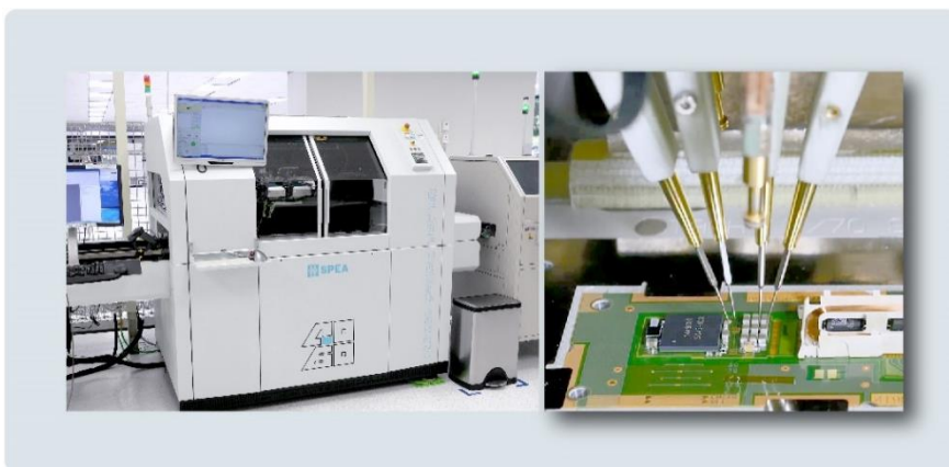
Figure 9. The MSEI production test suite and monitoring system uses electrical testers like the FPT shown on the left. The right-most image depicts the tester probing a capacitor.
