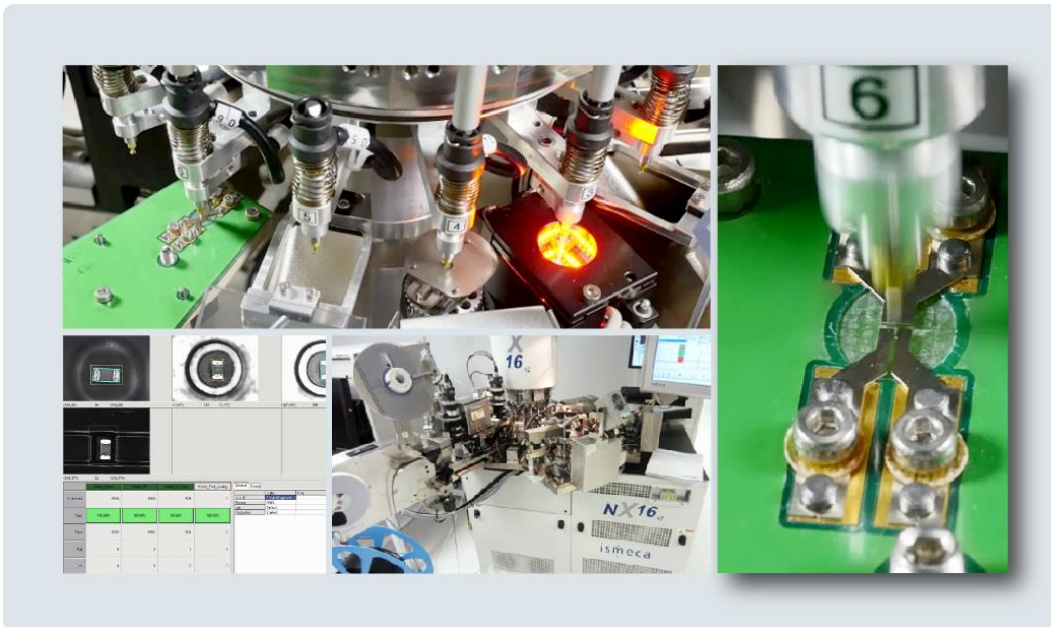
Figure 5. MSEI's automated capacitor test, handling, and tape and reel machine
