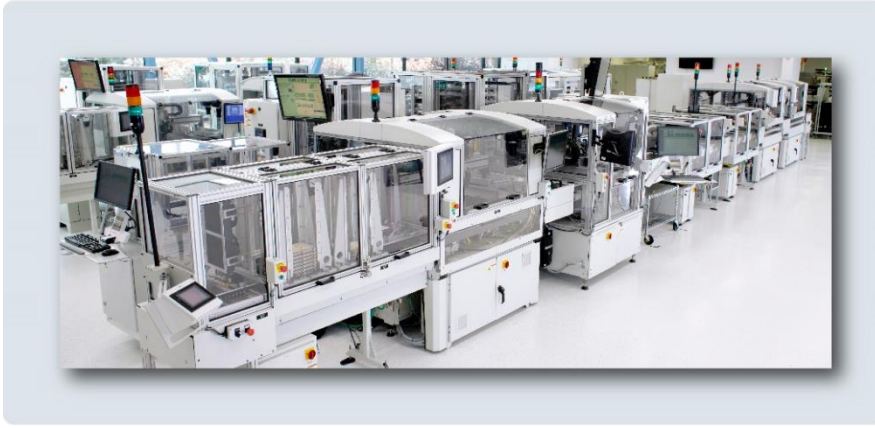
Figure 10. The AFTS handles all module functional tests during production
