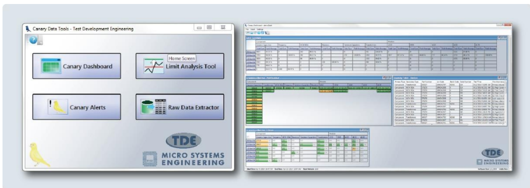
Figure 7. MSEI’s software suite provides simultaneous background analysis and alert generation of multiple components types, parts and lots. The lots highlighted in yellow on the right indicate observations that require further investigation prior to acceptance
